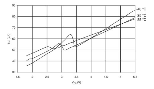
Figure 31-231. ATmega168A: AREF External Reference Current vs.  $V_{\rm CC}$
