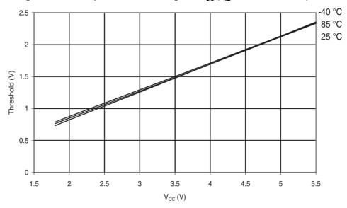
Figure 31-219. ATmega168A: Reset Pin Input Hysteresis vs.  $V_{\rm CC}$
