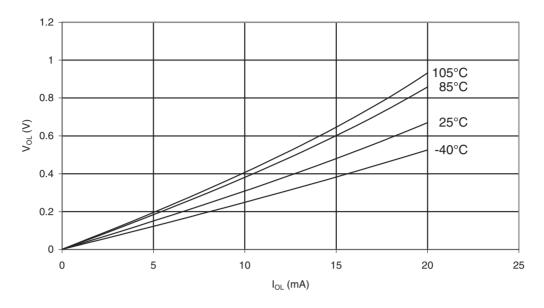
Figure 33-21.ATmega88PA: I/O Pin Output Voltage vs. Sink Current (V<sub>CC</sub> = 5V)
