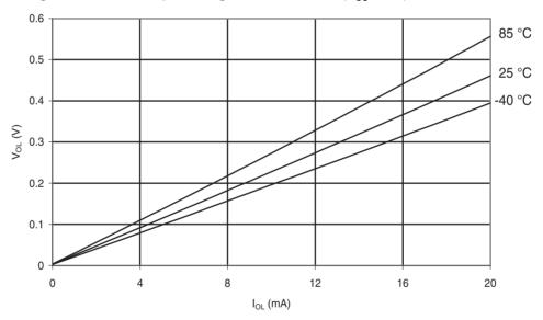
Figure 31-212. ATmega168A: I/O Pin Output Voltage vs. Source Current (Vcc = 3 V)
