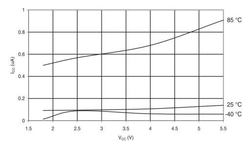
Figure 31-201. ATmega168A: Power-Down Supply Current vs. V<sub>CC</sub> (Watchdog Timer Enabled)
