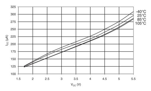
Figure 34-42.ATmega168PA: Analog Comparator Current vs. V<sub>CC</sub>
