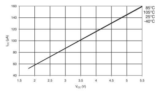
Figure 35-41.ATmega328P: Analog Comparator Current vs. V<sub>CC</sub>
