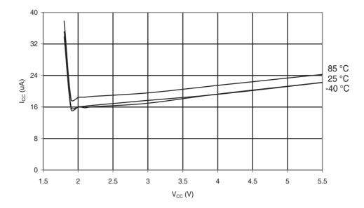
Figure 31-44. ATmega48A: Programming Current vs. V<sub>CC</sub>
