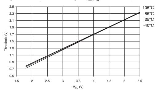
Figure 35-30.ATmega328P: Reset Pin Input Hysteresis vs. V<sub>CC</sub>
