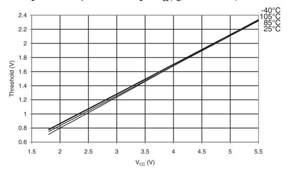
Figure 32-29.ATmega48PA: Reset Pin Input Hysteresis vs.  $V_{\rm CC}$
