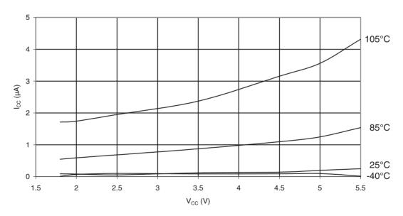
Figure 33-12.ATmega88PA: Power-Down Supply Current vs. V<sub>CC</sub> (Watchdog Timer Enabled)
