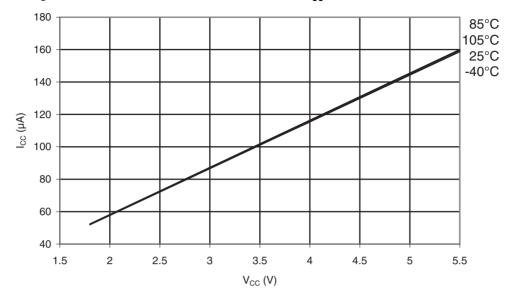
Figure 35-43.ATmega328P: Brownout Detector Current vs. V<sub>CC</sub>
