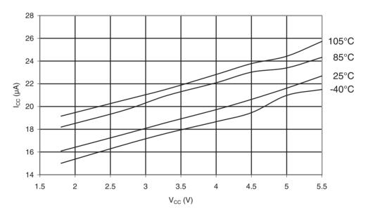
Figure 31-281. ATmega168PA: Programming Current vs. V<sub>CC</sub>
