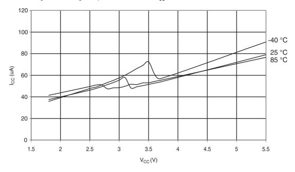
Figure 31-326. ATmega328: AREF External Reference Current vs.  $V_{\rm CC}$
