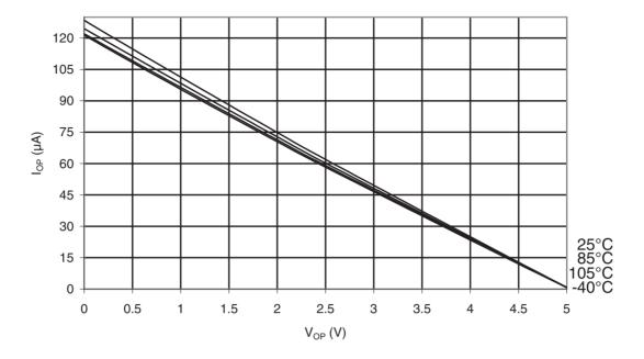
Figure 31-65. ATmega48PA: Reset Pull-up Resistor Current vs. Reset Pin Voltage (V<sub>CC</sub> = 1.8V)
