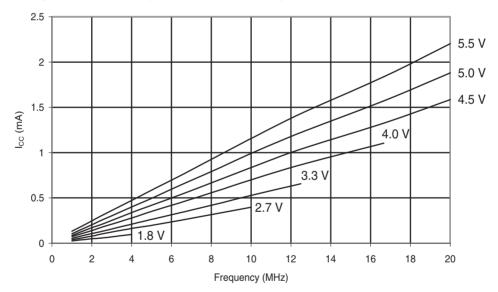
Figure 31-149. ATmega88PA: Idle Supply Current vs. V<sub>CC</sub> (Internal RC Oscillator, 128kHz)
