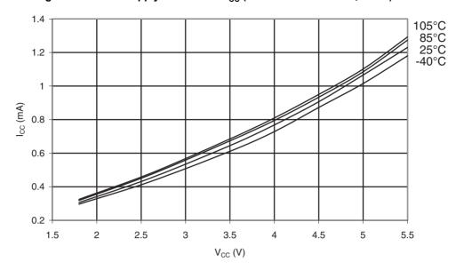
Figure 31-336. ATmega328P: Active Supply Current vs.  $V_{CC}$  (Internal RC Oscillator, 8MHz)
