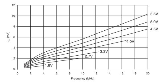
Figure 33-3. ATmega88PA: Active Supply Current vs. V<sub>CC</sub> (Internal RC Oscillator, 128kHz)
