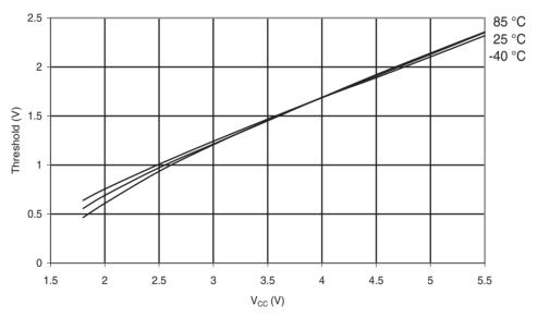
Figure 31-27. ATmega48A: I/O Pin Input Hysteresis vs.  $V_{\rm CC}$
