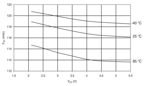
Figure 31-226. ATmega168A: Calibrated 8MHz RC Oscillator Frequency vs. V<sub>CC</sub>
