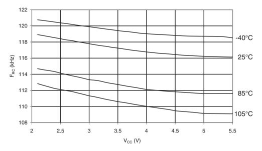
Figure 31-274. ATmega168PA: Calibrated 8MHz RC Oscillator Frequency vs. V<sub>CC</sub>
