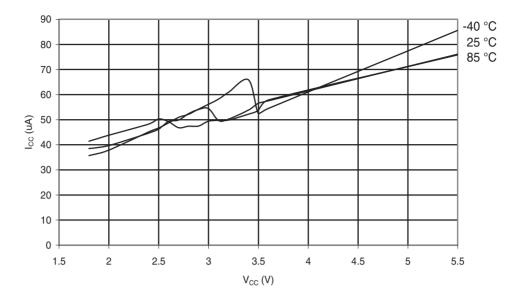
Figure 31-42. ATmega48A: AREF External Reference Current vs. V<sub>CC</sub>
