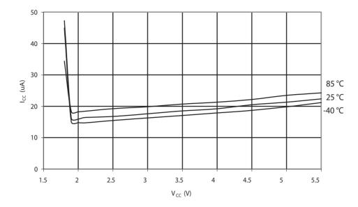
Figure 31-138. ATmega88A: Programming Current vs. V<sub>CC</sub>
