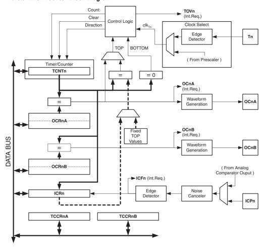
Figure 16-1. 16-bit Timer/Counter Block Diagram<sup>(1)</sup>
