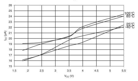
Figure 32-42.ATmega48PA: Programming Current vs. V<sub>CC</sub>
