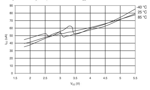
Figure 31-136. ATmega88A: AREF External Reference Current vs. V<sub>CC</sub>
