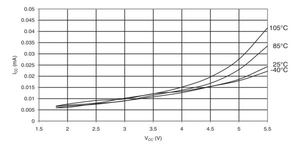
Figure 33-9. ATmega88PA: Idle Supply Current vs. V<sub>CC</sub> (Internal RC Oscillator, 1MHz)
