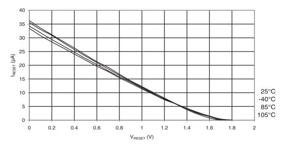
Figure 31-160. ATmega88PA: Reset Pull-up Resistor Current vs. Reset Pin Voltage (V<sub>CC</sub> = 2.7V)
