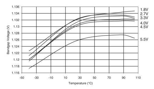
Figure 31-271. ATmega168PA: Calibrated Bandgap Voltage vs. Vcc
