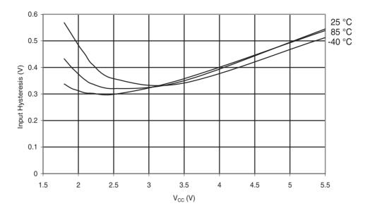
Figure 31-28. ATmega48A: Reset Input Threshold Voltage vs. V<sub>CC</sub> (V<sub>IH</sub>, I/O Pin read as '1)'
