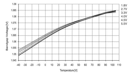
Figure 31-176. ATmega88PA: Bandgap Voltage vs. V<sub>CC</sub>
