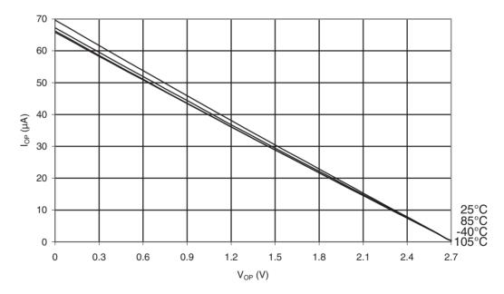
Figure 32-16.ATmega48PA: I/O Pin Pull-up Resistor Current vs. Input Voltage ( $V_{CC} = 5V$ )
