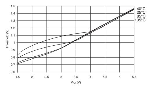
Figure 31-265. ATmega168PA: Reset Input Threshold Voltage vs. V<sub>CC</sub> (V<sub>IL</sub>, I/O Pin read as '0')
