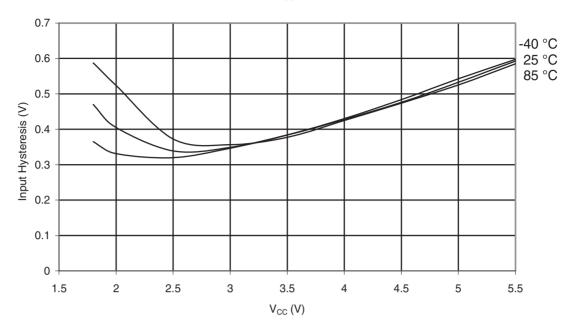
Figure 31-312. ATmega328: Reset Input Threshold Voltage vs. V<sub>CC</sub> (V<sub>IH</sub>, I/O Pin read as '1')
