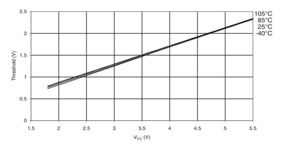
Figure 33-29.ATmega88PA: Reset Pin Input Hysteresis vs.  $V_{\rm CC}$
