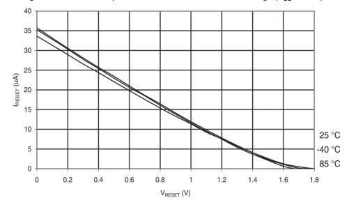
Figure 31-208. ATmega168A: Reset Pull-up Resistor Current vs. Reset Pin Voltage ( $V_{CC} = 2.7 \text{ V}$ )
