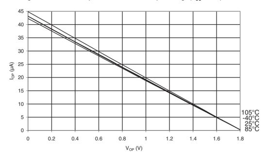
Figure 32-15.ATmega48PA: I/O Pin Pull-up Resistor Current vs. Input Voltage ( $V_{CC} = 2.7V$ )
