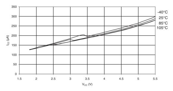
Figure 33-39.ATmega88PA: Analog Comparator Current vs. V<sub>CC</sub>
