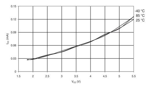
Figure 31-193. ATmega168A: Active Supply Current vs. V<sub>CC</sub> (Internal RC Oscillator, 1MHz)
