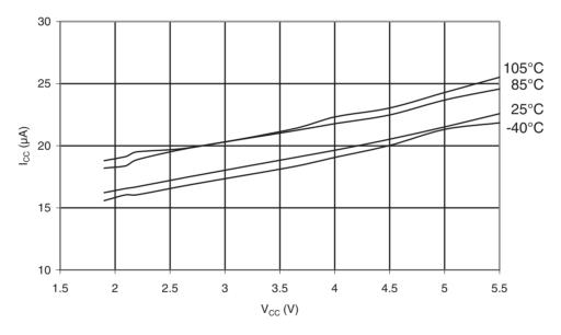
Figure 31-375. ATmega328P: Programming Current vs. V<sub>CC</sub>
