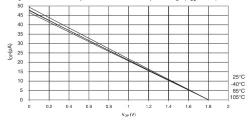
Figure 35-16.ATmega328P: I/O Pin Pull-up Resistor Current vs. Input Voltage ( $V_{CC} = 2.7V$ )
