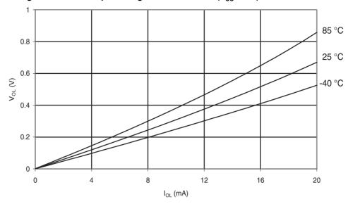
Figure 31-116. ATmega88A: I/O Pin Output Voltage vs. Sink Current (V<sub>CC</sub> = 5 V)
