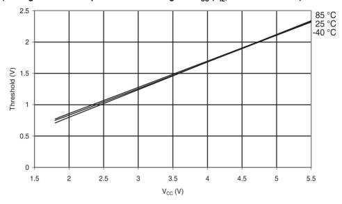
Figure 31-30. ATmega48A: Reset Pin Input Hysteresis vs.  $V_{\rm CC}$
