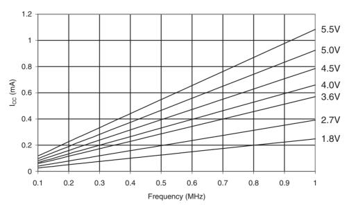
Figure 31-333. ATmega328P: Active Supply Current vs. Frequency (1-20MHz)
