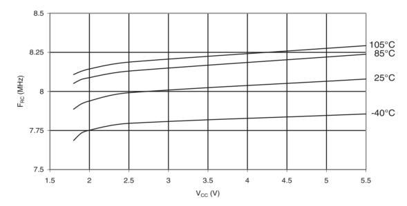
Figure 33-36.ATmega88PA: Calibrated 8MHz RC Oscillator Frequency vs. Temperature
