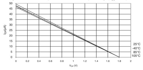
Figure 31-347. ATmega328P: I/O Pin Pull-up Resistor Current vs. Input Voltage ( $V_{CC} = 2.7V$ )
