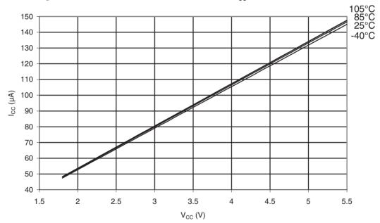
Figure 31-90. ATmega48PA: Brownout Detector Current vs. V<sub>CC</sub>
