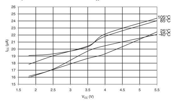
Figure 31-91. ATmega48PA: Programming Current vs. V<sub>CC</sub>
