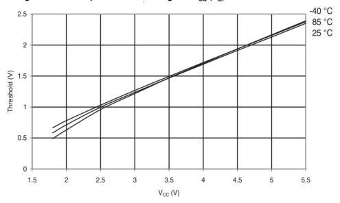
Figure 31-121. ATmega88A: I/O Pin Input Hysteresis vs. V<sub>CC</sub>
