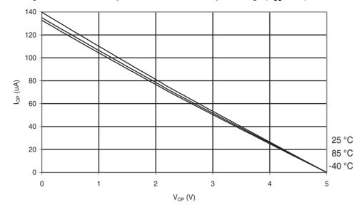
Figure 31-112. ATmega88A: Reset Pull-up Resistor Current vs. Reset Pin Voltage (V<sub>CC</sub> = 1.8 V)
