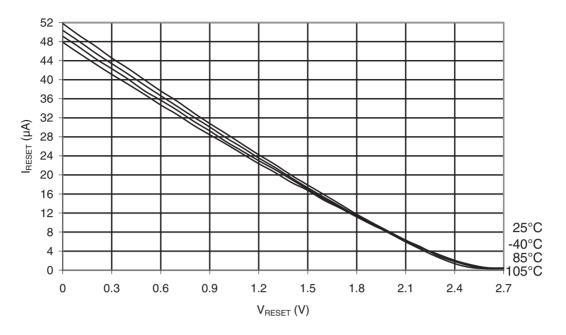
Figure 31-67. ATmega48PA: Reset Pull-up Resistor Current vs. Reset Pin Voltage (V<sub>CC</sub> = 5V)
