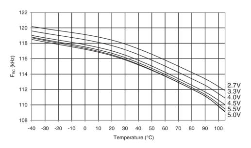
Figure 31-273. ATmega168PA: Watchdog Oscillator Frequency vs. V<sub>CC</sub>
