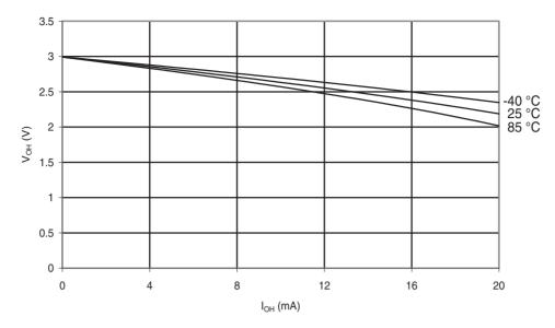
Figure 31-213. ATmega168A: I/O Pin Output Voltage vs. Source Current ( $V_{CC} = 5 V$ )
