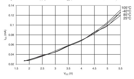
Figure 34-4. ATmega168PA: Active Supply Current vs. V<sub>CC</sub> (Internal RC Oscillator, 1MHz)
