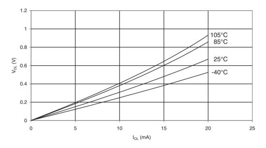
Figure 31-163. ATmega88PA: I/O Pin Output Voltage vs. Sink Current (V<sub>CC</sub> = 5V)
