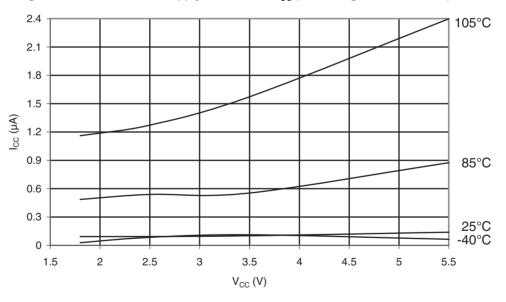
Figure 34-12.ATmega168PA: Power-Down Supply Current vs. V<sub>CC</sub> (Watchdog Timer Enabled)
