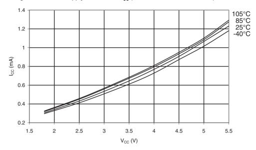
Figure 35-5. ATmega328P: Active Supply Current vs. V<sub>CC</sub> (Internal RC Oscillator, 8MHz)
