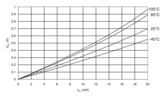
Figure 31-69. ATmega48PA: I/O Pin Output Voltage vs. Sink Current (V<sub>CC</sub> = 5V)
