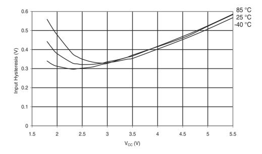
Figure 31-217. ATmega168A: Reset Input Threshold Voltage vs. V<sub>CC</sub> (V<sub>IH</sub>, I/O Pin read as '1')
