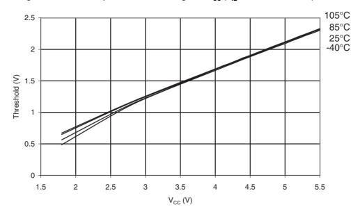
Figure 34-27.ATmega168PA: I/O Pin Input Hysteresis vs.  $V_{\rm CC}$
