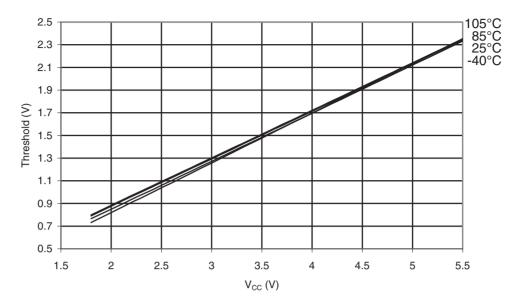
Figure 31-266. ATmega168PA: Reset Pin Input Hysteresis vs.  $V_{\rm CC}$
