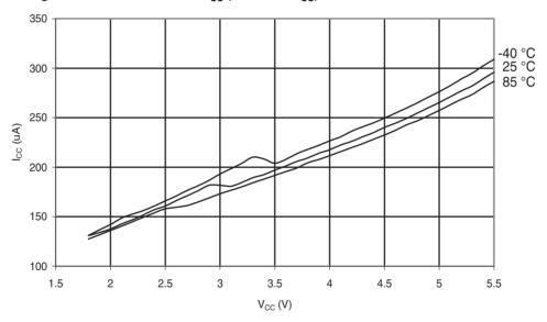
Figure 31-230. ATmega168A: Analog Comparator Current vs. V<sub>CC</sub>
