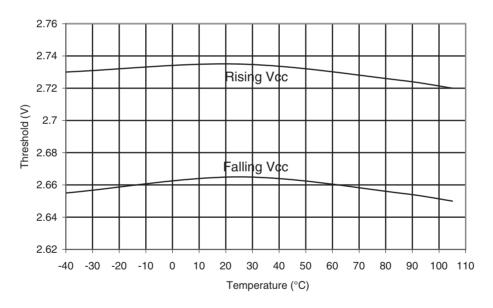
Figure 31-269. ATmega168PA: BOD Thresholds vs. Temperature (BODLEVEL is 4.3V)
