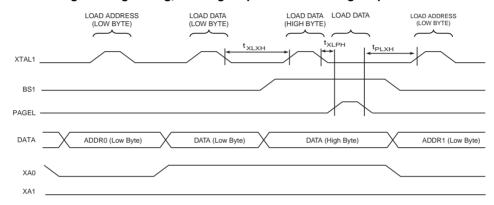
Note: 1. The timing requirements shown in Figure 29-6 (i.e.,  $t_{DVXH}$ ,  $t_{XHXL}$ , and  $t_{XLDX}$ ) also apply to loading operation.
