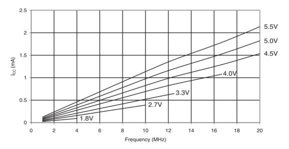
Figure 33-8. ATmega88PA: Idle Supply Current vs. V<sub>CC</sub> (Internal RC Oscillator, 128kHz)
