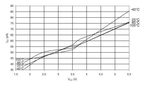
Figure 31-89. ATmega48PA: AREF External Reference Current vs. V<sub>CC</sub>
