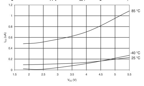
Figure 31-12. ATmega48A: Power-Down Supply Current vs. V<sub>CC</sub> (Watchdog Timer Enabled)
