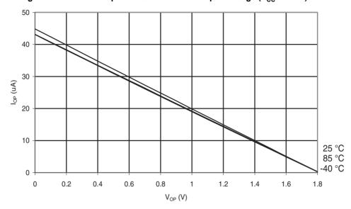
Figure 31-16. ATmega48A: I/O Pin Pull-up Resistor Current vs. Input Voltage (V<sub>CC</sub> = 2.7 V)
