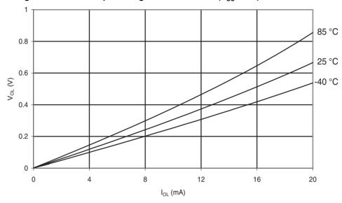
Figure 31-211. ATmega168A: I/O Pin Output Voltage vs. Sink Current (V<sub>CC</sub> = 5 V)
