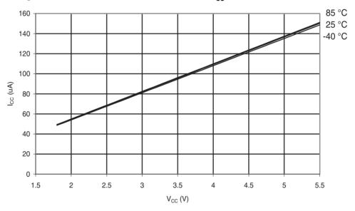
Figure 31-137. ATmega88A: Brownout Detector Current vs. V<sub>CC</sub>
