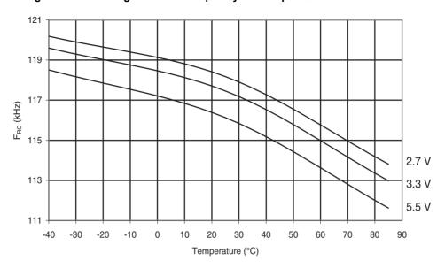
Figure 31-225. ATmega168A: Watchdog Oscillator Frequency vs. V<sub>CC</sub>
