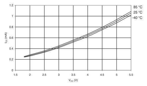
Figure 31-194. ATmega168A: Active Supply Current vs. V<sub>CC</sub> (Internal RC Oscillator, 8MHz)
