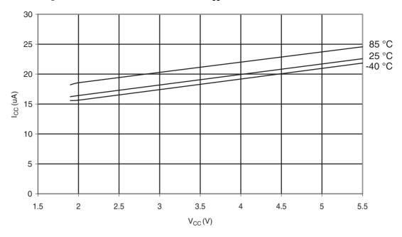
Figure 31-328. ATmega328: Programming Current vs. V<sub>CC</sub>
