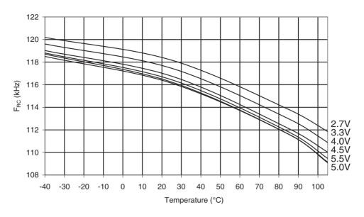
Figure 34-37.ATmega168PA: Watchdog Oscillator Frequency vs. V<sub>CC</sub>
