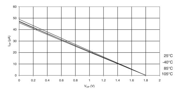
Figure 31-157. ATmega88PA: I/O Pin Pull-up Resistor Current vs. Input Voltage ( $V_{CC} = 2.7V$ )
