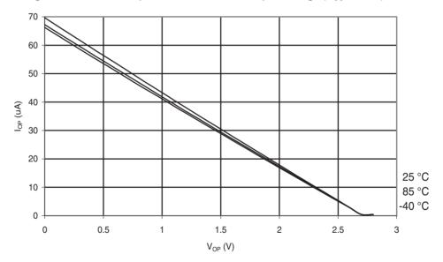
Figure 31-17. ATmega48A: I/O Pin Pull-up Resistor Current vs. Input Voltage ( $V_{CC} = 5V$ )
