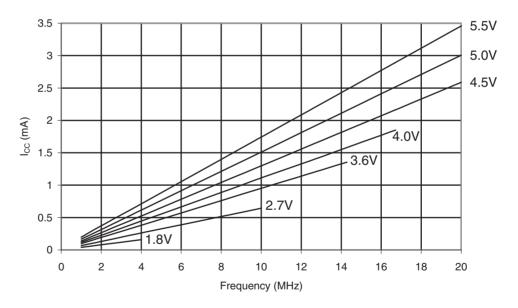
Figure 31-339. ATmega328P: Idle Supply Current vs. V<sub>CC</sub> (Internal RC Oscillator, 128kHz)
