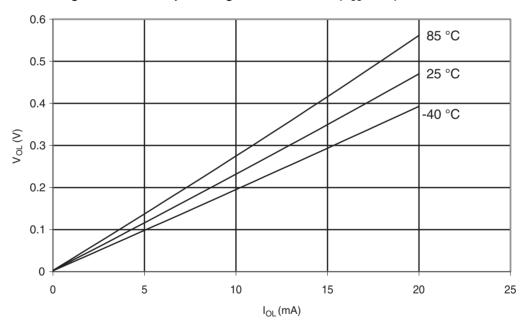
Figure 31-307. ATmega328: I/O Pin Output Voltage vs. Source Current (Vcc = 3 V)
