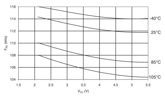
Figure 31-84. ATmega48PA: Calibrated 8MHz RC Oscillator Frequency vs.  $V_{\rm CC}$
