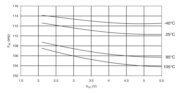
Figure 33-35.ATmega88PA: Calibrated 8MHz RC Oscillator Frequency vs.  $V_{\text{CC}}$
