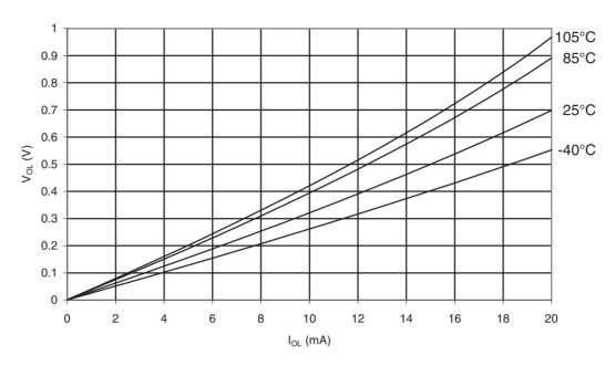
Figure 32-21.ATmega48PA: I/O Pin Output Voltage vs. Sink Current (V<sub>CC</sub> = 5V)
