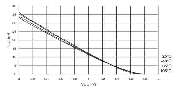
Figure 33-18.ATmega88PA: Reset Pull-up Resistor Current vs. Reset Pin Voltage ( $V_{CC} = 2.7V$ )
