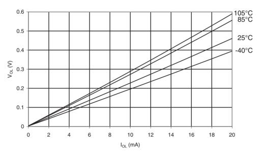
Figure 31-259. ATmega168PA: I/O Pin Output Voltage vs. Source Current (V<sub>CC</sub> = 3V)
