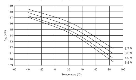
Figure 31-320. ATmega328: Watchdog Oscillator Frequency vs. V<sub>CC</sub>
