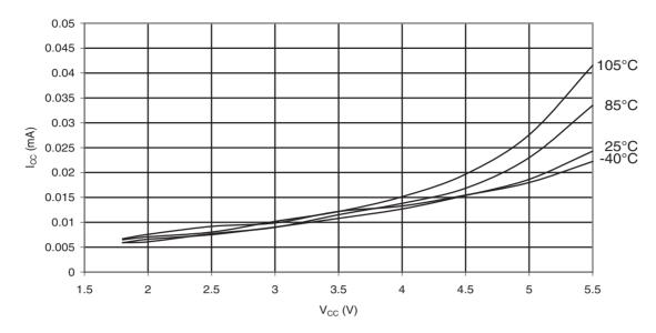
Figure 31-150. ATmega88PA: Idle Supply Current vs. V<sub>CC</sub> (Internal RC Oscillator, 1MHz)
