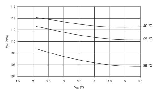
Figure 31-131. ATmega88A: Calibrated 8MHz RC Oscillator Frequency vs. V<sub>CC</sub>
