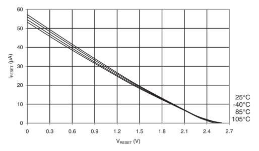
Figure 31-351. ATmega328P: Reset Pull-up Resistor Current vs. Reset Pin Voltage (V<sub>CC</sub> = 5V)
