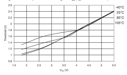
Figure 35-29.ATmega328P: Reset Input Threshold Voltage vs.  $V_{CC}$  ( $V_{IL}$ , I/O Pin read as '0')
