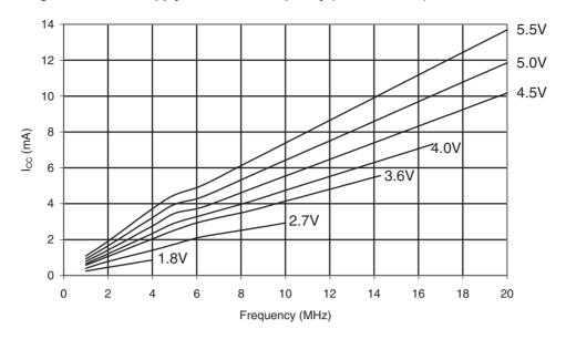
Figure 35-3. ATmega328P: Active Supply Current vs.  $V_{CC}$  (Internal RC Oscillator, 128kHz)
