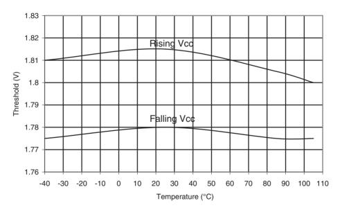
Figure 34-32.ATmega168PA: BOD Thresholds vs. Temperature (BODLEVEL is 2.7V)
