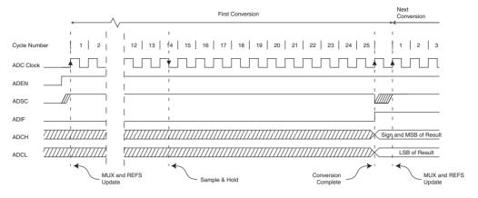
Figure 24-5. ADC Timing Diagram, Single Conversion
