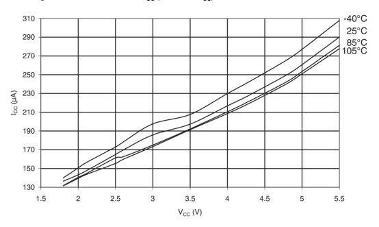
Figure 32-39.ATmega48PA: Analog Comparator Current vs.  $V_{\text{CC}}$
