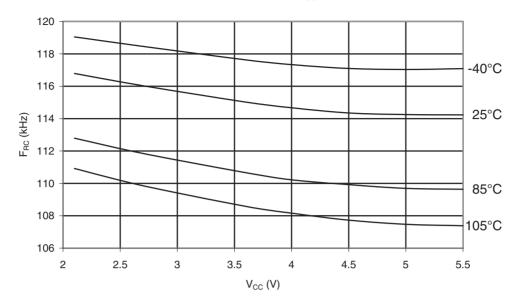
Figure 35-37.ATmega328P: Calibrated 8 MHz RC Oscillator Frequency vs.  $V_{CC}$
