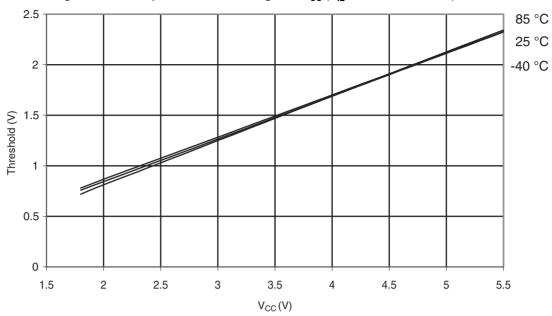
Figure 31-314. ATmega328: Reset Pin Input Hysteresis vs.  $V_{\rm CC}$
