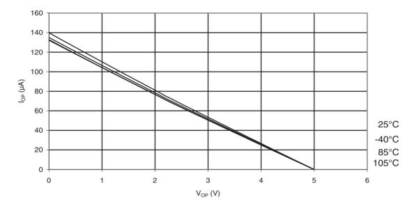
Figure 31-159. ATmega88PA: Reset Pull-up Resistor Current vs. Reset Pin Voltage (V<sub>CC</sub> = 1.8V)
