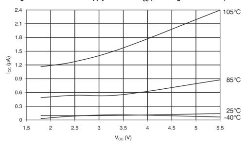
Figure 31-248. ATmega168PA: Power-Down Supply Current vs. V<sub>CC</sub> (Watchdog Timer Enabled)
