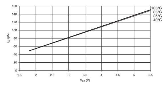
Figure 33-41.ATmega88PA: Brownout Detector Current vs. V<sub>CC</sub>
