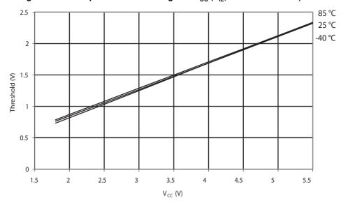
Figure 31-124. ATmega88A: Reset Pin Input Hysteresis vs.  $V_{\rm CC}$
