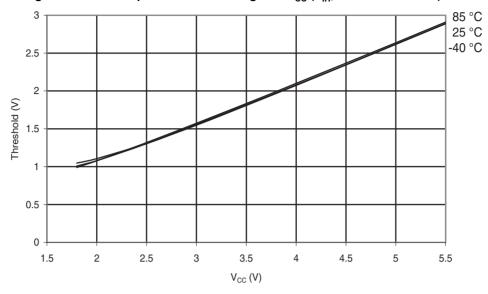
Figure 31-215. ATmega168A: I/O Pin Input Threshold Voltage vs. V<sub>CC</sub> (V<sub>IL</sub>, I/O Pin read as '0')
