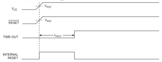
Figure 11-3. MCU Start-up, RESET Extended Externally
