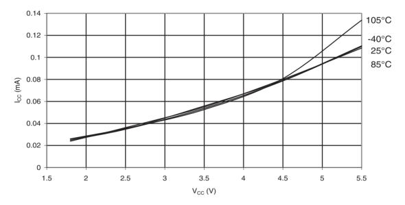
Figure 33-4. ATmega88PA: Active Supply Current vs. V<sub>CC</sub> (Internal RC Oscillator, 1MHz)
