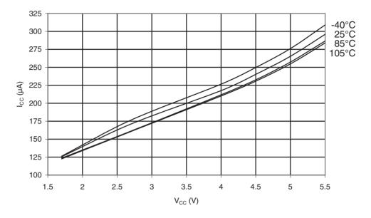
Figure 31-278. ATmega168PA: Analog Comparator Current vs. V<sub>CC</sub>
