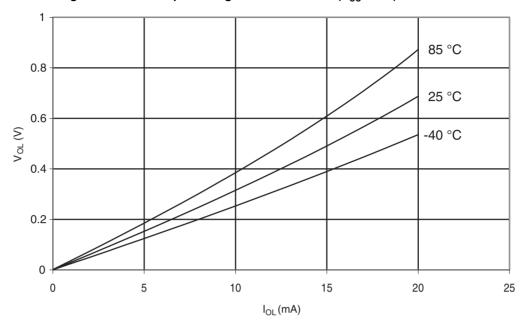
Figure 31-306. ATmega328: I/O Pin Output Voltage vs. Sink Current (V<sub>CC</sub> = 5 V)
