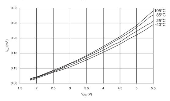
Figure 32-10.ATmega48PA: Idle Supply Current vs. Vcc (Internal RC Oscillator, 8MHz)
