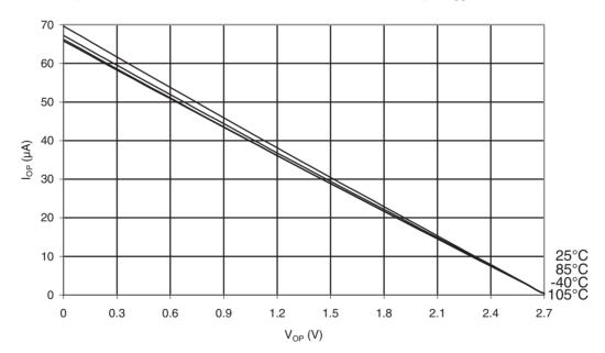
Figure 31-64. ATmega48PA: I/O Pin Pull-up Resistor Current vs. Input Voltage ( $V_{CC} = 5V$ )
