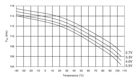
Figure 32-34.ATmega48PA: Watchdog Oscillator Frequency vs. V<sub>CC</sub>
