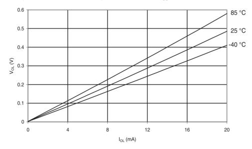
Figure 31-23. ATmega48A: I/O Pin Output Voltage vs. Source Current (Vcc = 3 V)
