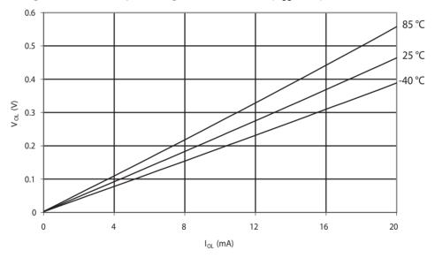
Figure 31-117. ATmega88A: I/O Pin Output Voltage vs. Source Current (Vcc = 3 V)
