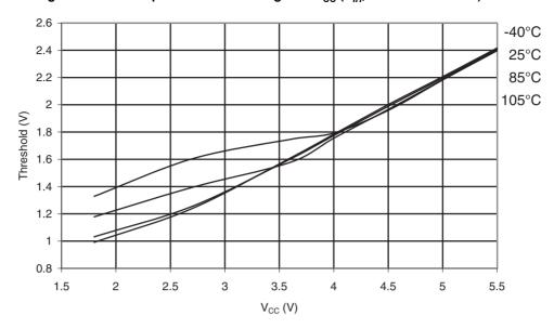
Figure 31-360. ATmega328P: Reset Input Threshold Voltage vs.  $V_{CC}$  ( $V_{IL}$ , I/O Pin read as '0')
