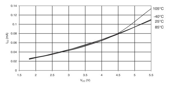
Figure 31-145. ATmega88PA: Active Supply Current vs. V<sub>CC</sub> (Internal RC Oscillator, 1MHz)
