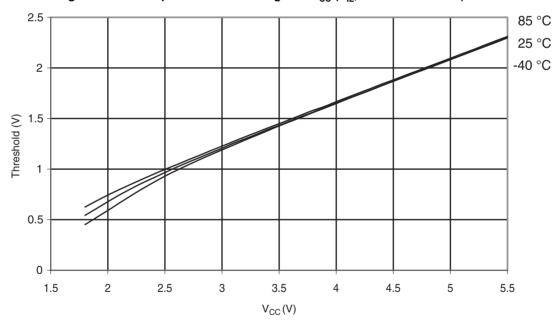
Figure 31-311. ATmega328: I/O Pin Input Hysteresis vs. V<sub>CC</sub>
