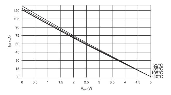
Figure 32-17.ATmega48PA: Reset Pull-up Resistor Current vs. Reset Pin Voltage (V<sub>CC</sub> = 1.8V)
