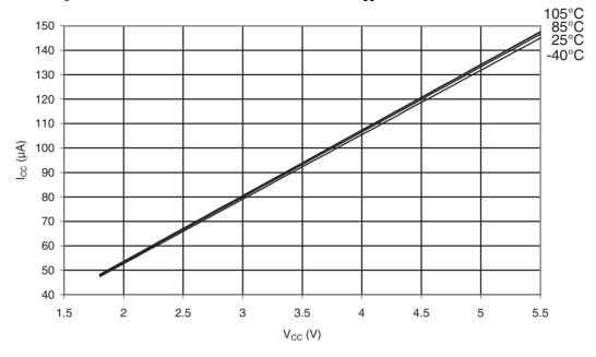
Figure 32-41.ATmega48PA: Brownout Detector Current vs.  $V_{CC}$
