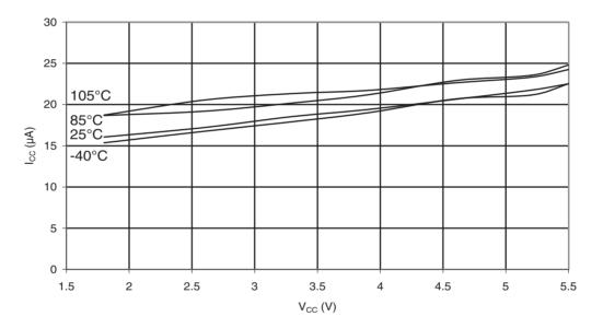
Figure 31-186. ATmega88PA: Programming Current vs. V<sub>CC</sub>
