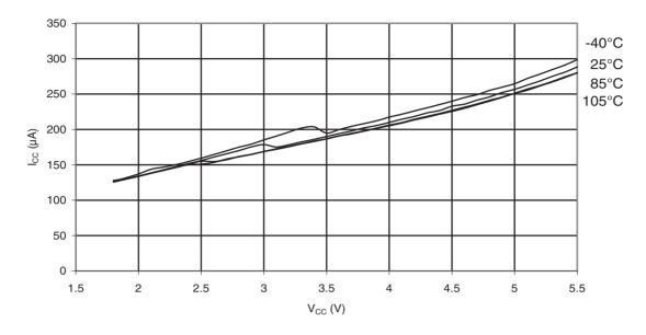
Figure 31-183. ATmega88PA: Analog Comparator Current vs.  $V_{\rm CC}$
