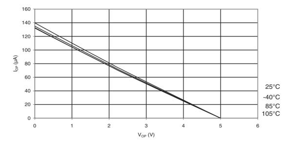
Figure 33-17.ATmega88PA: Reset Pull-up Resistor Current vs. Reset Pin Voltage (V<sub>CC</sub> = 1.8V)
