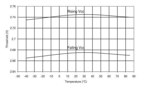
Figure 31-127. ATmega88A: BOD Thresholds vs. Temperature (BODLEVEL is 4.3 V)
