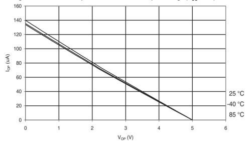
Figure 31-207. ATmega168A: Reset Pull-up Resistor Current vs. Reset Pin Voltage (V<sub>CC</sub> = 1.8 V)
