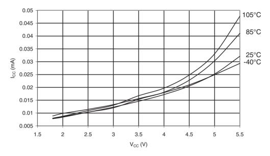
Figure 31-340. ATmega328P: Idle Supply Current vs. V<sub>CC</sub> (Internal RC Oscillator, 1MHz)
