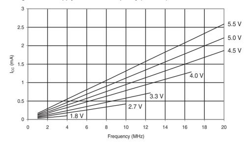
Figure 31-8. ATmega48A: Idle Supply Current vs. V<sub>CC</sub> (Internal RC Oscillator, 128kHz)
