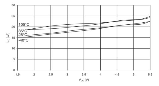
Figure 33-42.ATmega88PA: Programming Current vs. V<sub>CC</sub>
