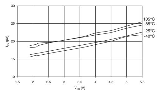
Figure 35-44.ATmega328P: Programming Current vs. V<sub>CC</sub>
