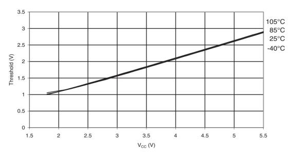
Figure 33-25.ATmega88PA: I/O Pin Input Threshold Voltage vs.  $V_{CC}$  ( $V_{IL}$ , I/O Pin read as '0')
