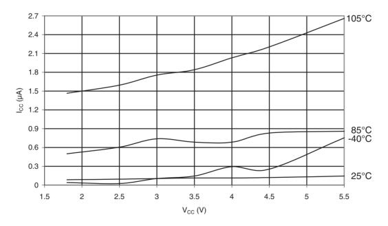
Figure 32-12.ATmega48PA: Power-Down Supply Current vs. V<sub>CC</sub> (Watchdog Timer Enabled)
