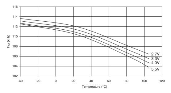
Figure 33-34.ATmega88PA: Watchdog Oscillator Frequency vs. V<sub>CC</sub>
