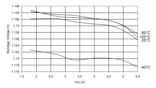
Figure 34-35.ATmega168PA: Calibrated Bandgap Voltage vs. Temperature
