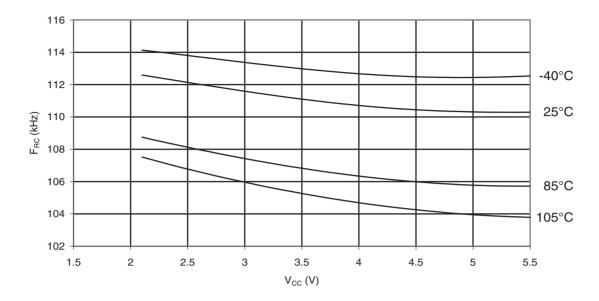
Figure 31-179. ATmega88PA: Calibrated 8MHz RC Oscillator Frequency vs.  $V_{\text{CC}}$
