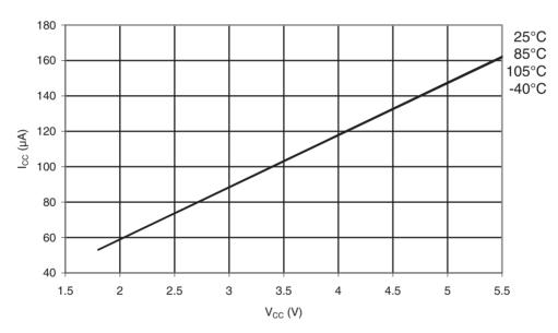
Figure 34-44.ATmega168PA: Brownout Detector Current vs. V<sub>CC</sub>
