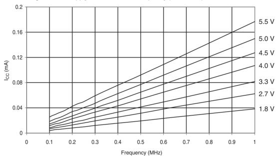
Figure 31-291. ATmega328: Idle Supply Current vs. Frequency (1-20MHz)
