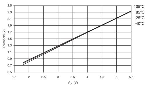
Figure 31-361. ATmega328P: Reset Pin Input Hysteresis vs. V<sub>CC</sub>
