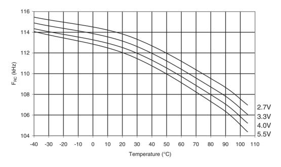
Figure 31-83. ATmega48PA: Watchdog Oscillator Frequency vs. V<sub>CC</sub>
