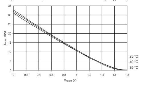
Figure 31-19. ATmega48A: Reset Pull-up Resistor Current vs. Reset Pin Voltage ( $V_{CC} = 2.7 \text{ V}$ )
