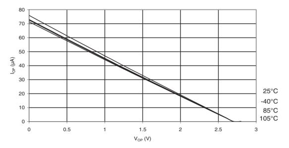
Figure 31-158. ATmega88PA: I/O Pin Pull-up Resistor Current vs. Input Voltage ( $V_{CC} = 5V$ )
