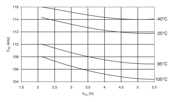
Figure 32-35.ATmega48PA: Calibrated 8MHz RC Oscillator Frequency vs.  $V_{\text{CC}}$
