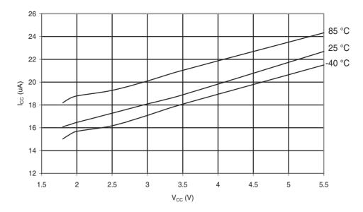
Figure 31-233. ATmega168A: Programming Current vs. V<sub>CC</sub>
