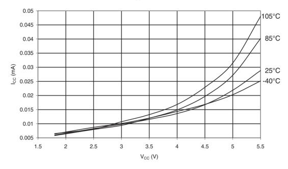
Figure 32-9. ATmega48PA: Idle Supply Current vs. V<sub>CC</sub> (Internal RC Oscillator, 1MHz)
