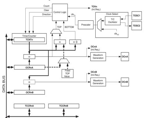
Figure 18-1. 8-bit Timer/Counter Block Diagram
