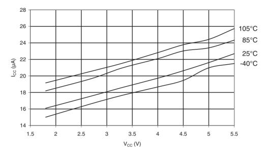
Figure 34-45.ATmega168PA: Programming Current vs. V<sub>CC</sub>
