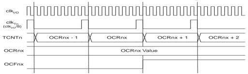
Figure 18-11 shows the setting of OCF2A and the clearing of TCNT2 in CTC mode.
