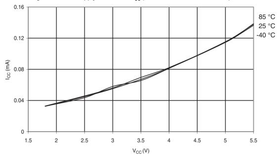
Figure 31-288. ATmega328: Active Supply Current vs.  $V_{CC}$  (Internal RC Oscillator, 1MHz)
