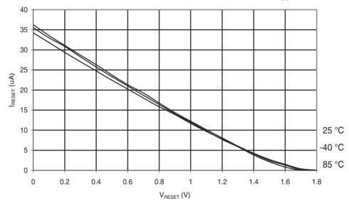
Figure 31-113. ATmega88A: Reset Pull-up Resistor Current vs. Reset Pin Voltage ( $V_{CC} = 2.7 \text{ V}$ )
