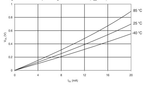
Figure 31-22. ATmega48A: I/O Pin Output Voltage vs. Sink Current ( $V_{CC} = 5 V$ )
