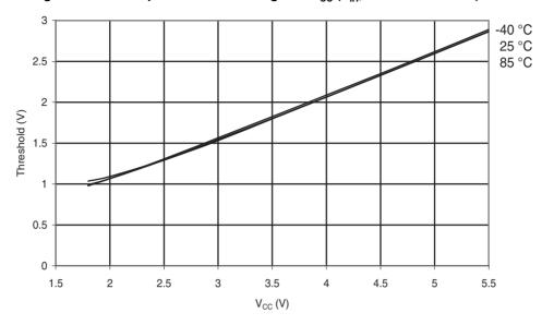
Figure 31-26. ATmega48A: I/O Pin Input Threshold Voltage vs.  $V_{CC}$  ( $V_{IL}$ , I/O Pin read as '0')
