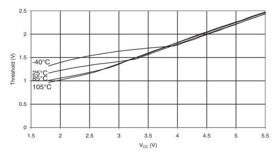
Figure 31-170. ATmega88PA: Reset Input Threshold Voltage vs. V<sub>CC</sub> (V<sub>IL</sub>, I/O Pin read as '0')
